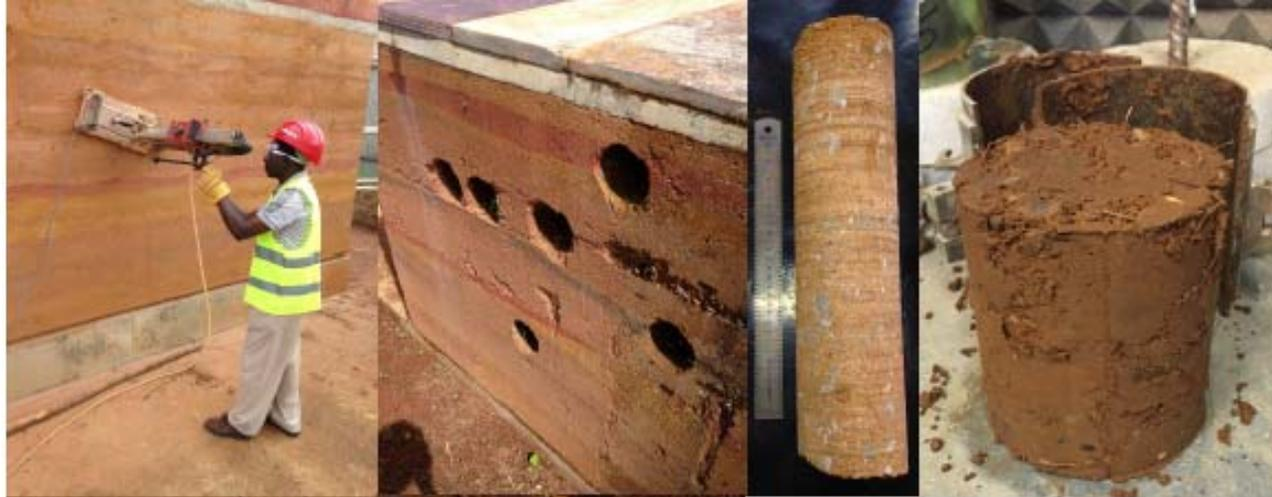
Abrasion resistance test and non-destructive surveys
